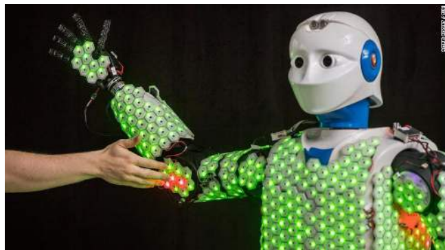
Figure 13: High resolution Robot skin being developed for expanding the scope of Robotics
