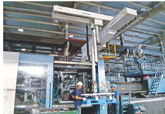
Figure 21: Robots are being used in loading and unloading
